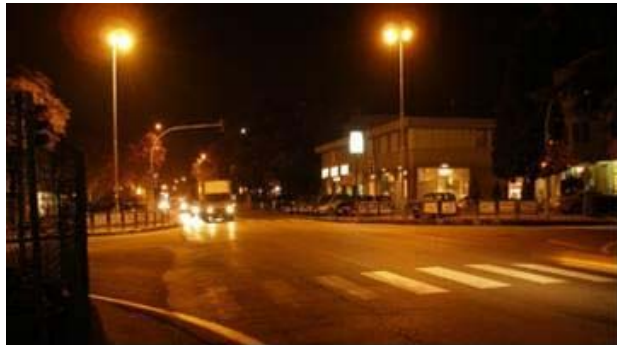
High Pressure Sodium
